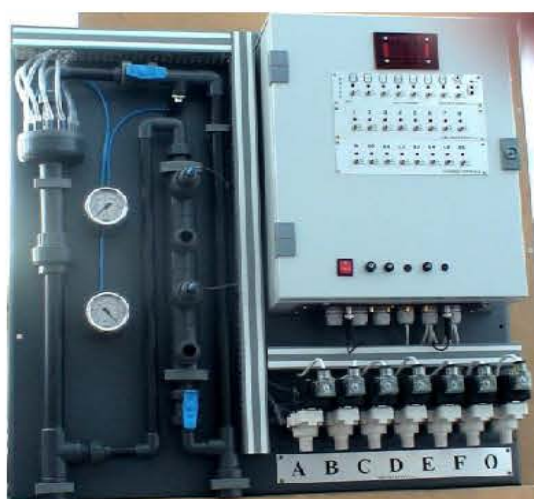
壁挂式 CAUA-6 型水肥一体化营养液自动调控装备 Wall-mounted integrated water and fertilizer automatic control equipment
